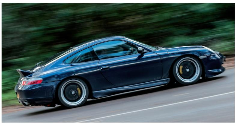
Mark McConnell's RPM modified C4 has a massive spec with a rebuilt engine, using Hartech liners, plus lightweight flywheel and sports exhaust and headers. Suspension is Bilstein PSS10 and GT3 geometry
